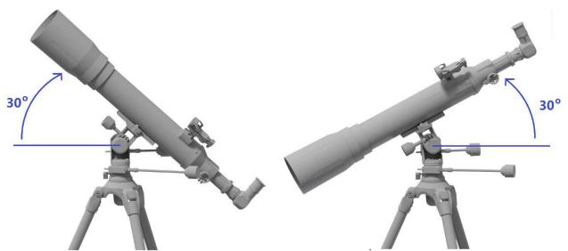
**Altitude limit.** This range, of around -30 to +30 degrees, allows the OTA to remain more or less balanced to the mount, even if the centre of gravity is a bit off.
