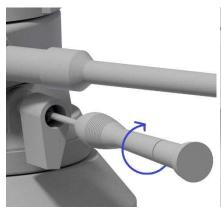
While pulled-out, use a screwdriver (Philips-type) and tighten the inner screw.
