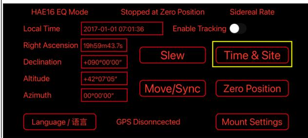
Click on **Time & Site**, then tap on **Sync Current Device Time to Mount** and **Sync Current Device Location to Mount** to set the mount Time and Site info.
