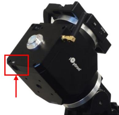
10. **Mount control via a SmartPhone/Tablet:** The mount can be controlled by the iOptron Commander Lite app for initial settings, as well as slew, GOTO and tracking.
