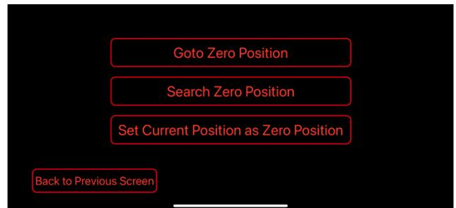
You may also perform this by click on **Zero Position =>Search Zero Position**, then press **ENTER**, if an optional 8411 handset is used. Follow the online instruction to complete the process. The Zero Position can be set via the 8411 handset, the iOptron Commander/Lite, or the planetarium software.
