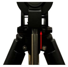
Install Counterweight(s): Before CW is installed, make sure the mount is at zero position, i.e., CW shaft points to the ground. Disengage the R.A. Gear Switch to set the R.A. axis free before loading the CW. Remove the CW Safety Cap at the end of CW Shaft. Guide the CW over the shaft with large opening side facing down. Tighten the CW Locking Screw to hold the CW in place. Place the Safety Cap back onto the shaft. Move the CW to the bottom of the CW shaft and tighten the CW locking Screw.
