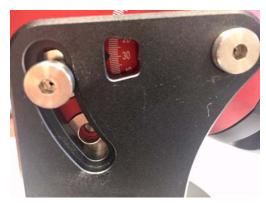
Remove the front Latitude Locking Screws and washers (one on each side) and thread them into high latitude position holes without tightening. Unthread and remove the Latitude Position Bolt.
