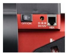
Plug GPS module into the iPORT with coiled cable. When power on, GPS ON sign should be displayed at the upper right corner of the hand controller.
