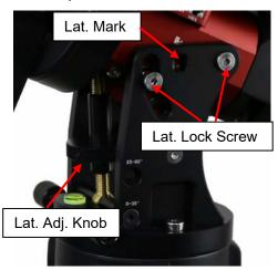
The mount can be set at  $0^{\sim}35^{\circ}$  (low latitude) or  $25^{\circ}$   $^{\sim}60^{\circ}$  (high latitude). To change the latitude setting from low to high, Latitude Position Bolt should be moved from  $0^{\sim}35^{\circ}$  to  $25^{\sim}60^{\circ}$  position, so as the Latitude Locking screws.
