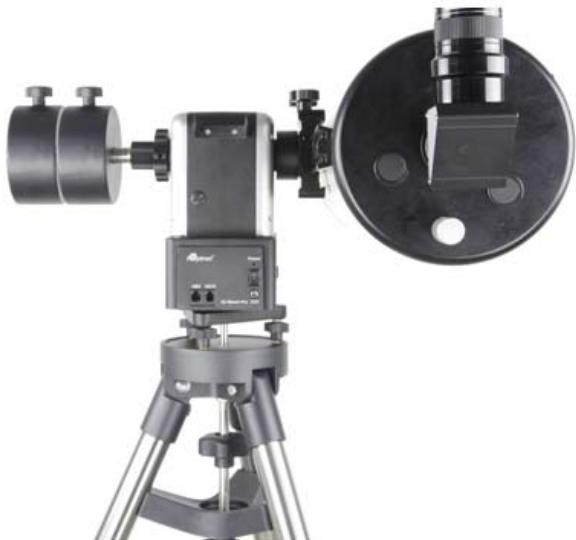
A simple and safe method to determine the CW and its position is by calculating the torques (*weight times the distance to the center*) of the payload and CW, and making them equal or close. Or shorten the front leg to adjust the balance: if the OTA side tends to swing, move the CW far out; *vice versa*.
