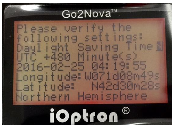
If all the information is correct, you may press **ENTER** to confirm and skip waiting for GPS signal. Or if the mount could not pick up the GPS signal (the mount won't advance to next step to start slewing), you can manually change it by setting Daylight Saving Time (DST) to Y(es) or N(o); adjusting the date and time; inputting your location
