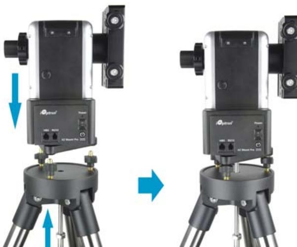
Thread the tripod bolt into the bottom of the mount while holding the mount with your hand. Slightly tighten the tripod bolt by turning the tripod bolt lock knob.
