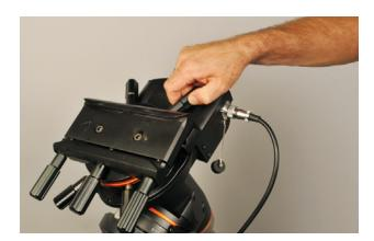
There are a total of eight clutch handles on the polar and declinations axes, as well as three more for clamping the Losmandystyle dovetail mounting saddle. While the handles provide positive locking, sometimes it can be difficult to get your hand around them because of tight clearances.
