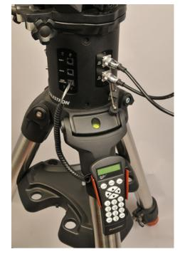
Most of the mount's electronics are housed in this 6-inch-diameter pier column. Cables for the drive motors, as well as the one for the external 12-volt DC power supply, use threaded connectors that prevent the cables from being accidentally pulled loose during use.
