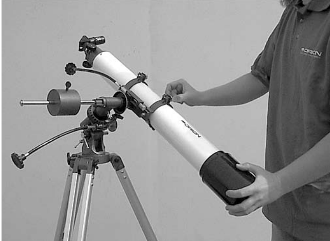
Figure 3d. Balancing the telescope with respect to the Dec. axis. As shown here, the telescope is out of balance (tilting).
