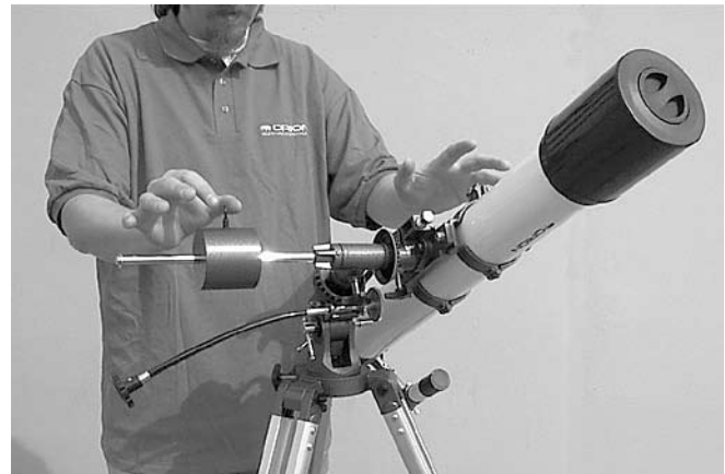
Figure 3b. Telescope is now balanced on the R.A. axis. That is, when hands are released, counterweight shaft remains horizontal.
