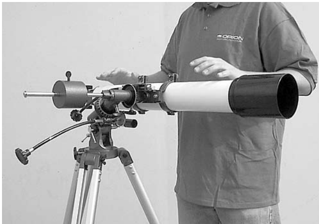
Figure 3e. Telescope is now balanced on the Dec. axis, i.e., it remains horizontal when hands are released.
